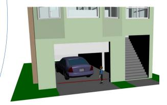
Flex IR with Microcell provides safety accross garage door openings to help prevent injuries from a closing garage door. The Flex IR protects the microcell from getting hit by cars or other heavy objects.
